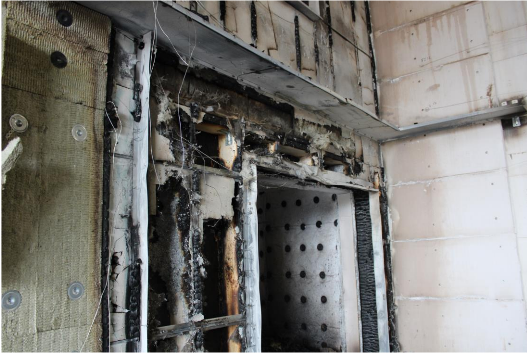
Photo No. 23 Test specimen after the test. Detailed photo below the first flame deflector
