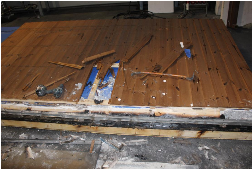
Photo No. 28 Test specimen after the test. Detailed photo of top prefabricated cassette. (charring on the lower formwork).
