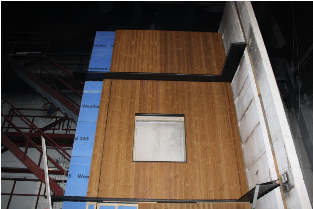
Photo No. 8 Vertical cladding was mounted. No cladding was mounted on the wing.
