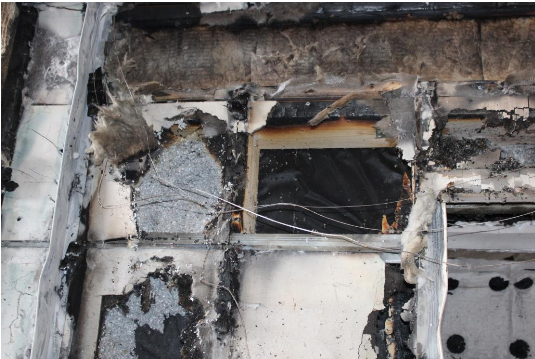
Photo No. 24 Test specimen after the test. Detailed photo of corner below the first flame deflector
