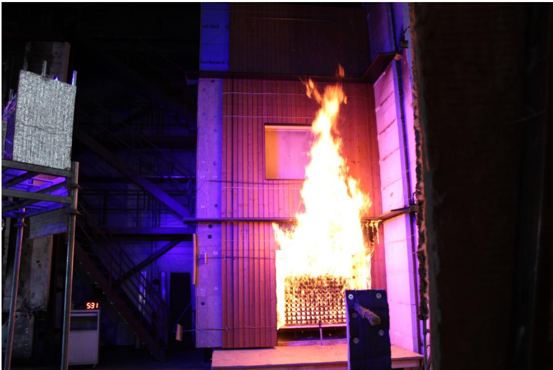
Photo No. 12 Test specimen 5 minutes into the test
