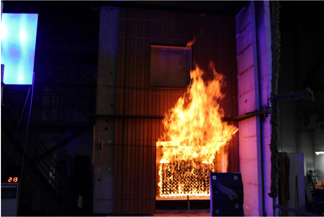
Photo No. 11 2 minutes into the test. Flames reaching first flame deflector.
