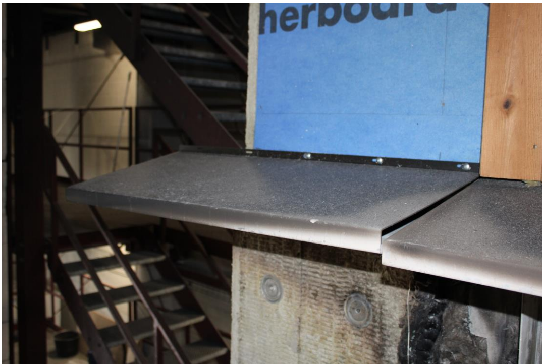
Photo No. 26 Test specimen after the test. Detailed photo of 2 nd flame deflector
